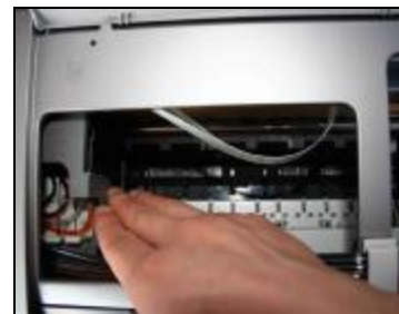
Make sure the length of tubeline is enough to reach the far left and right
